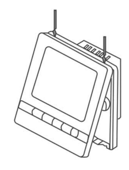
4. Hook the top part of the front cover on to the back plate and push the bottom part in to secure the fixture on the wall.
