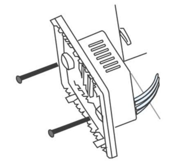
3. Use the screws provided to mount the thermostat on the wall.
