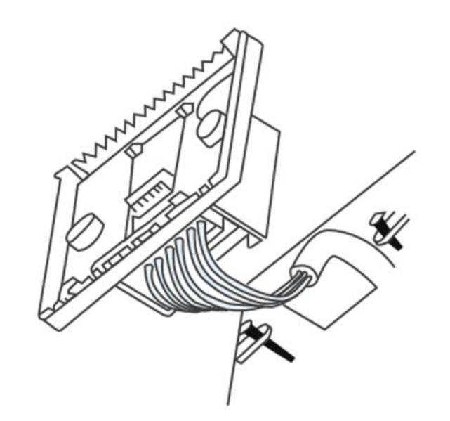
Connect the wires according to the wiring diagram, make sure they are tightly connected.
