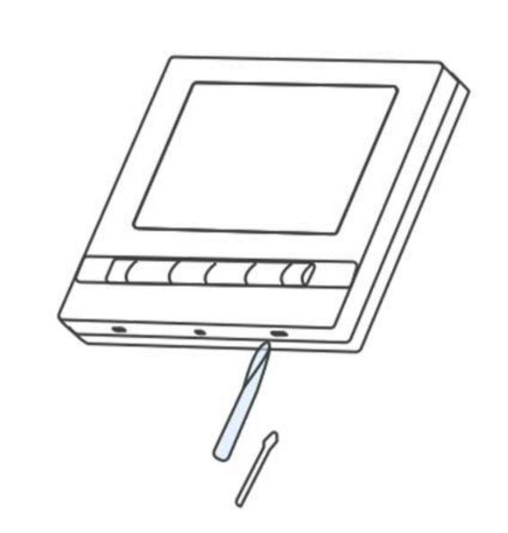
1. Use a flat screw driver to open the front cover of the thermostat.
